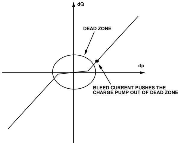
Figure 1. The Effect of Bleed Current on Charge Pump
