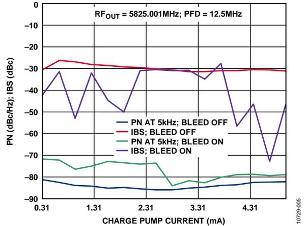
Figure 5. Phase Noise and IBS at 5825.001 MHz with a PFD Frequency = 12.5 MHz
