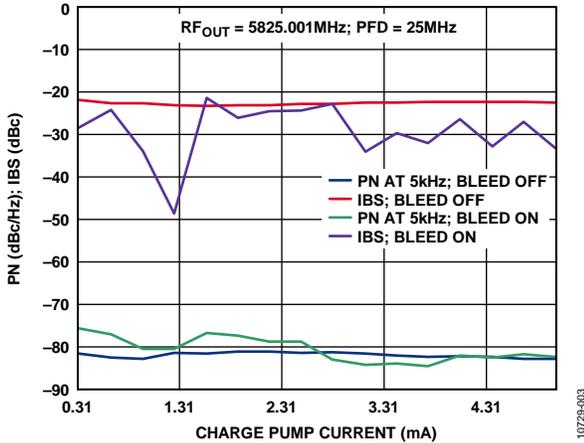
Figure 3. Phase Noise and IBS at 5825.001 MHz with a PFD Frequency = 25 MHz
