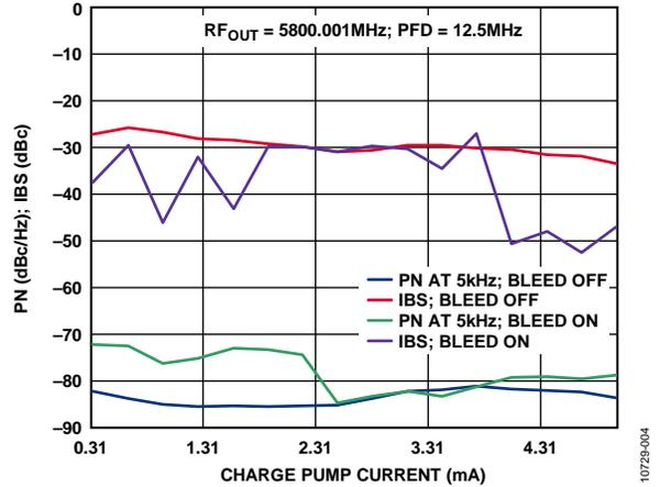
Figure 4. Phase Noise and IBS at 5800.001 MHz with a PFD Frequency = 12.5 MHz
