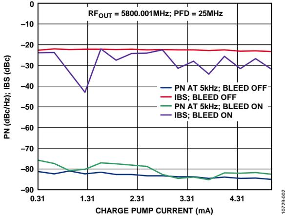
Figure 2. Phase Noise and IBS at 5800.001 MHz with a PFD Frequency = 25 MHz
