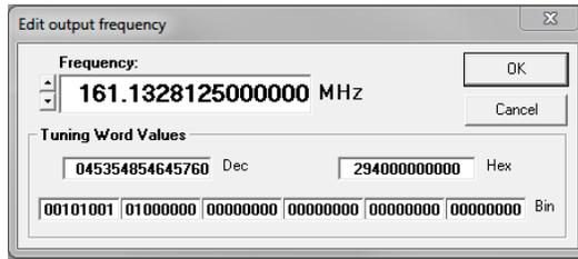
Figure 10. Edit Output Frequency Window
