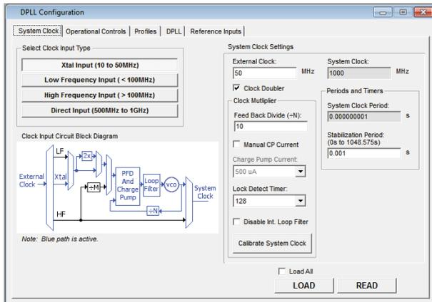
Figure 5. DPLL System Clock Configuration Window
