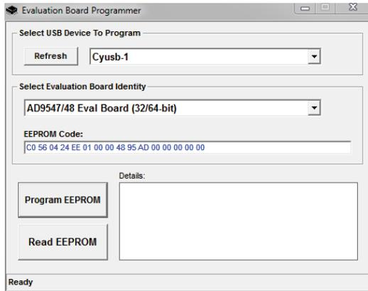
Figure 3. Evaluation Board USB Programmer
