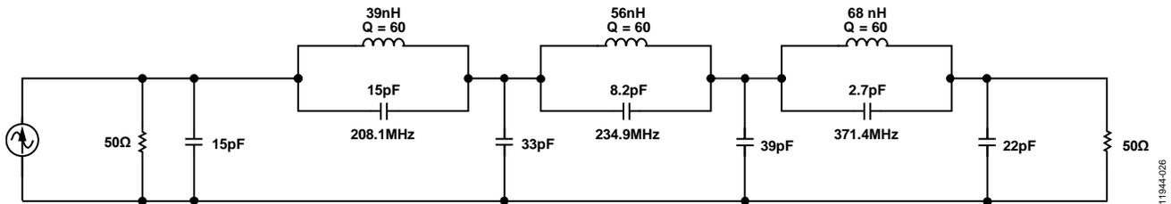
Figure 29. Evaluation Board Default Single-Ended Reconstruction Filter
