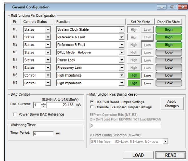
Figure 14. AD9548 General Configuration Window
