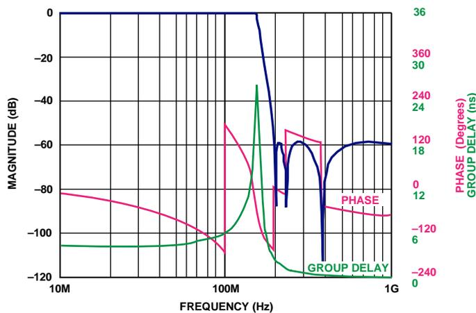
Figure 28. Frequency Response of Differential Reconstruction Filter Shown in Figure 25
