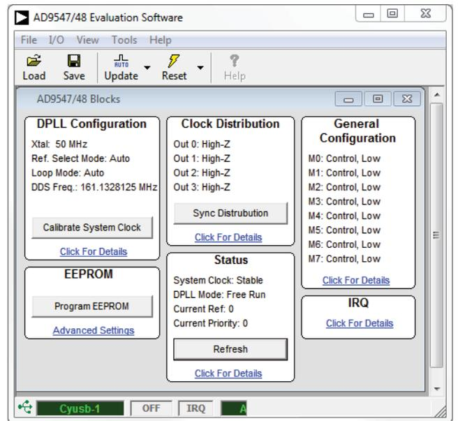
Figure 4. AD9548 Evaluation Software Main Window
