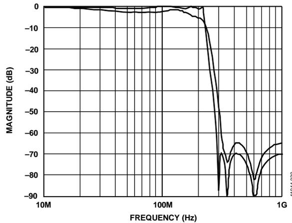
Figure 30. Frequency Response of Single-Ended Reconstruction Filter Shown in Figure 26
