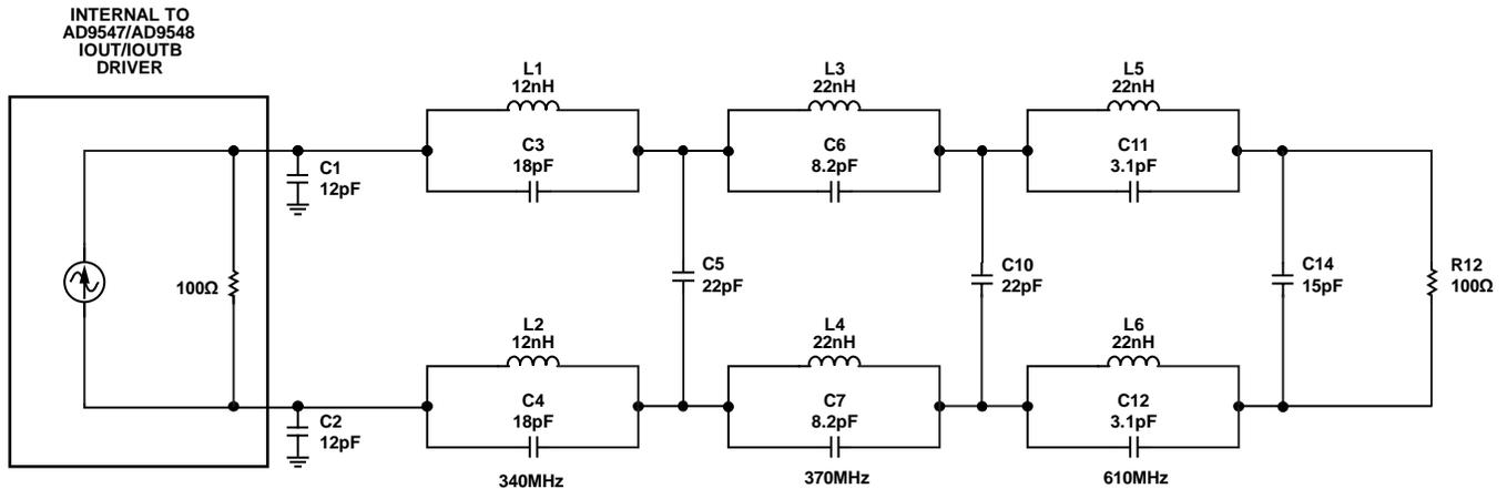
Figure 27. Default 240 MHz Differential Low-Pass Reconstruction Filter
