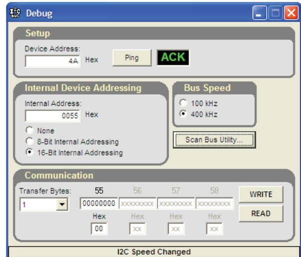
Figure 32. I<sup>2</sup>C Debug Window
