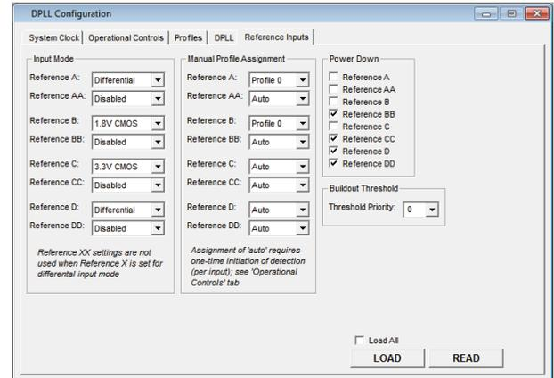
Figure 12. Reference Input Configuration Window
