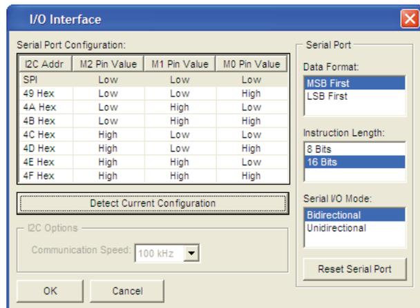
Figure 31. Serial Port Configuration
