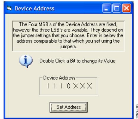
Figure 3. I<sup>2</sup>C Address Selection
