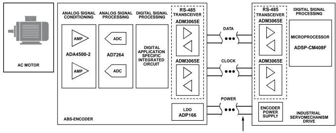
LONG CABLING (UP TO 150 METERS) BETWEEN THE MASTER INDUSTRIAL SERVOMECHANISM DRIVE AND SLAVE ABS-ENCODER 41 GR-001
