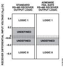
Figure 6. ADM3065E Receiver Fail-Safe Feature
