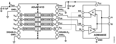
Figure 3. Signal Isolated 50 Mbps RS-485 Solution (Simplified Diagram – All Connections Not Shown)
