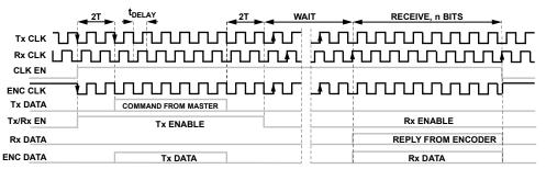
Figure 10. Timing Diagram for the Transmit/Receive Sequence
