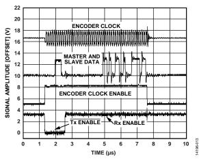
Figure 13. Control Lines During a Transmit and Receive Sequence
