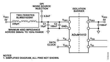
Figure 4. Typical Setup for DPI IEC 62132-4 Noise Immunity TEST
