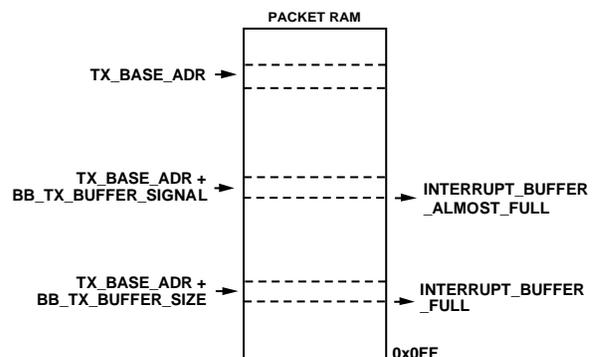
Figure 1. Rolling Buffer in Transmit Mode
