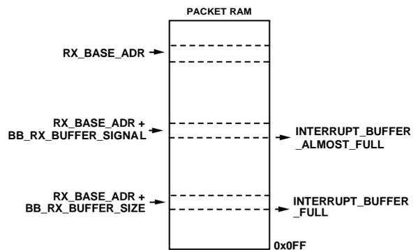
Figure 2. Rolling Buffer in Receive Mode
