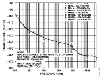
Figure 3. AD9523-1 Phase Noise, Output = 122.88 MHz (VCXO = 122.88 MHz, Crystek VCXO CVHD-950); Doubler On
