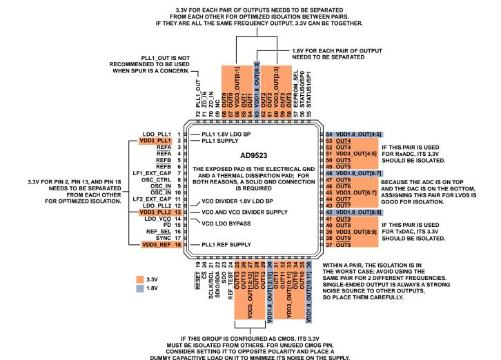
Figure 5. Power Supply Connections of the AD9523
