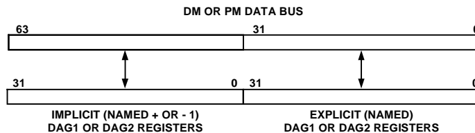
Figure 6-4: Long Word DAG Register-to-Data Register Transfers
