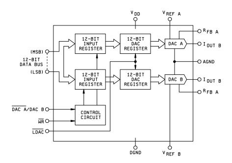
FIGURE 3. Functional diagram.
