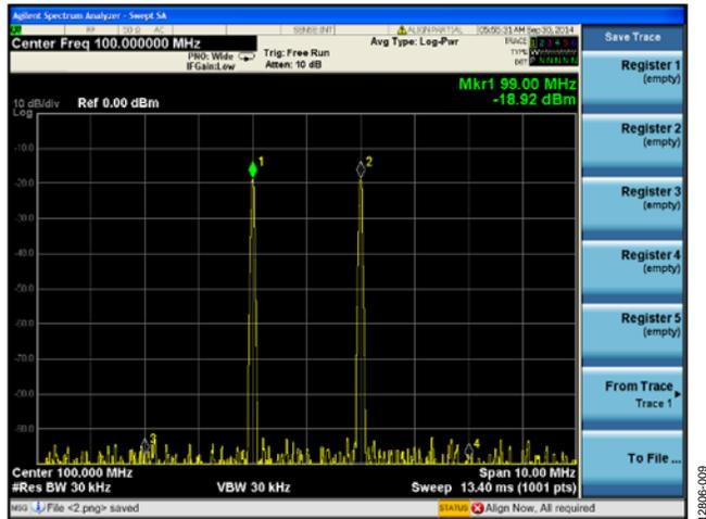
Figure 9. Spectrum Analyzer Display with ADA4961 Set to Maximum Gain
