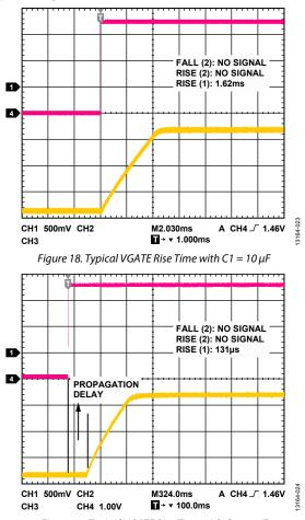
Figure 19. Typical VGATE Rise Time with  $C1 = 1 \mu F$
