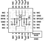
Figure 4. HMC1131 Multistage Externally Biased Amplifier
