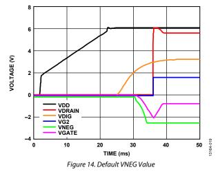
With the default configuration, the typical VGATE output swing is in between -2 V and 0 V. However,
