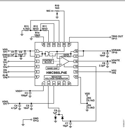
Figure 12. Typical Application Circuit for the HMC980LP4E
