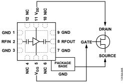
Figure 3. Typical Connections of an Externally Biased Amplifier
