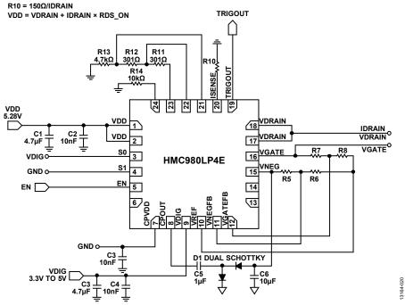
Figure 15. External Resistors for Adjusting Default VNEG and VGATE Values
