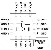
Figure 2. Typical Pinout for a Multistage Self Biased Amplifier with Multiple Bias Pins
