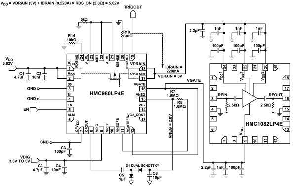
Figure 27. Application Circuit for Biasing the HMC1082LP4E with the HMC980LP4E
