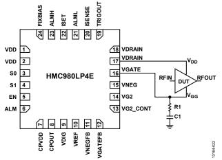
Figure 17. VGATE Connection Circuitry Between the HMC980LP4E and the DUT
