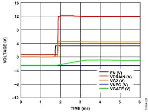
Figure 16. HMC980LP4E Typical Enable Waveform
