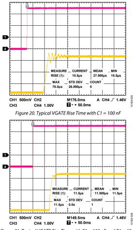
Figure 21. Typical VGATE Rise Time with C1 = 100 nF and R1 = 68  $\Omega$
