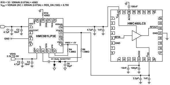
Figure 26. Application Circuit for Biasing the HMC460LC5 with the HMC981LP3E
