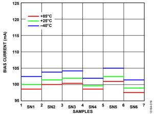
Figure 11. Improved Bias Current Variation of Same Amplifier when Biased with the HMC920LP5E
