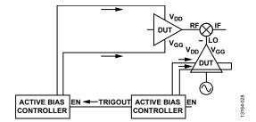
Figure 23. Daisy-Chain Configuration Where DUT Amplifiers Are on Different Signal Paths
