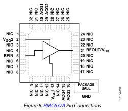
The amplifier provides 14 dB of gain, 43 dBm of output IP3, and 30.5 dBm of output power at a 1 dB gain compression under the bias conditions of  $V_{DD} = 12$  V,  $V_{GG}2 = 6$  V, and  $I_{DQ} = 400$  mA. The electrical specifications table of the HMC637A data sheet provides this information.
