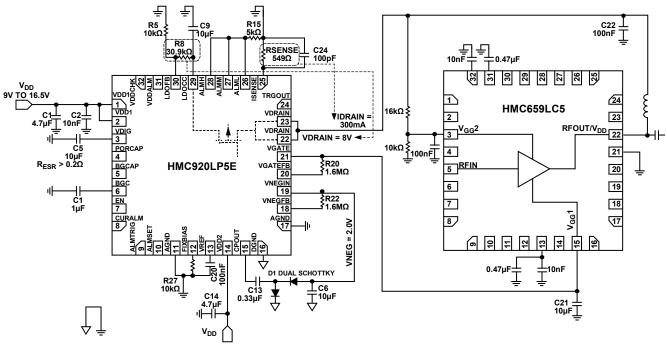
Figure 29. Application Circuit for Biasing the HMC659LC5 with the HMC920LP5E
