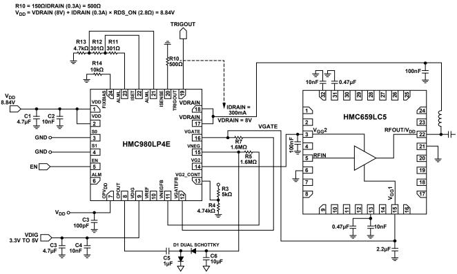
Figure 28. Application Circuit for Biasing the HMC659LC5 with the HMC980LP4E
