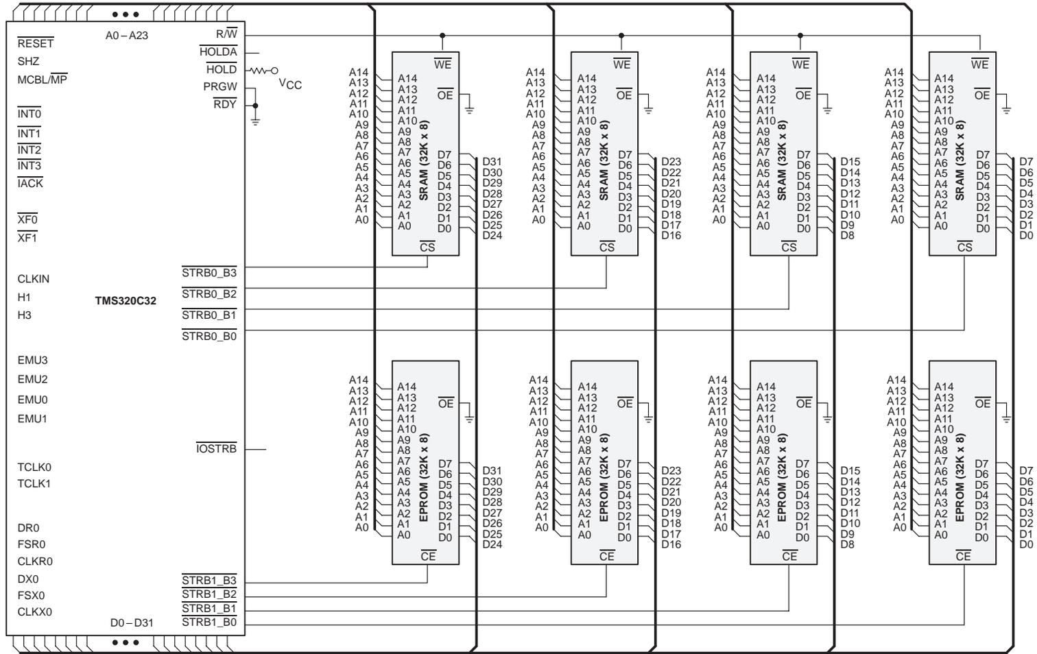
Figure 9. 32-Bit Memory Configuration ( $\overline{\text{STRB0}}$  and  $\overline{\text{STRB1}}$ )
