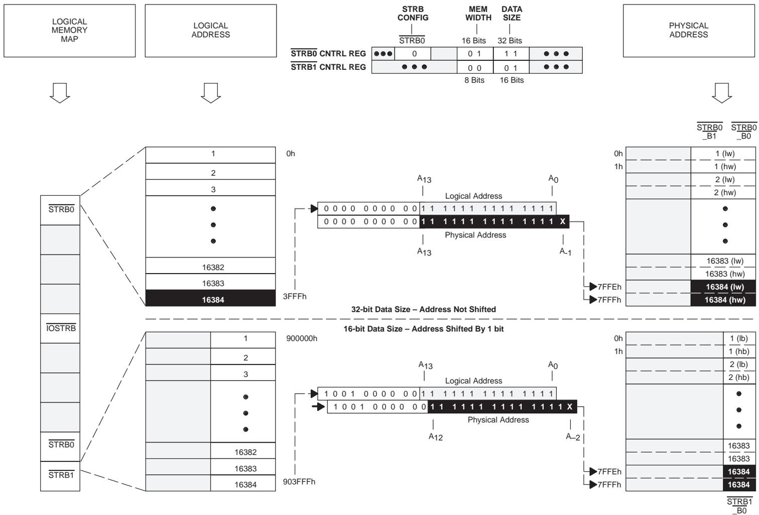
Figure 13. 16/8-Bit Memory Address Translation: Data Size > Memory Width
