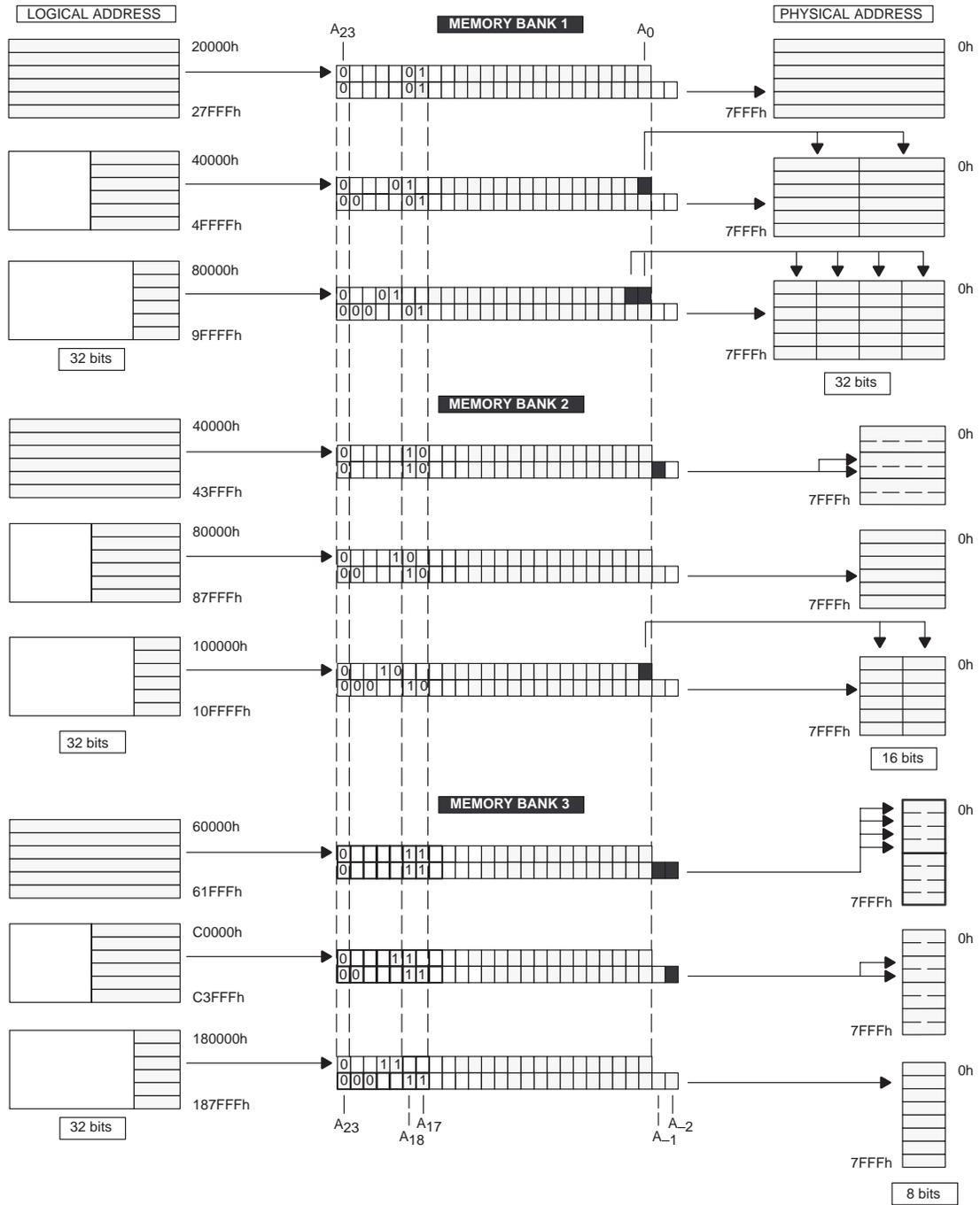
Figure 22. Address Decode for Multiple Memory Banks
