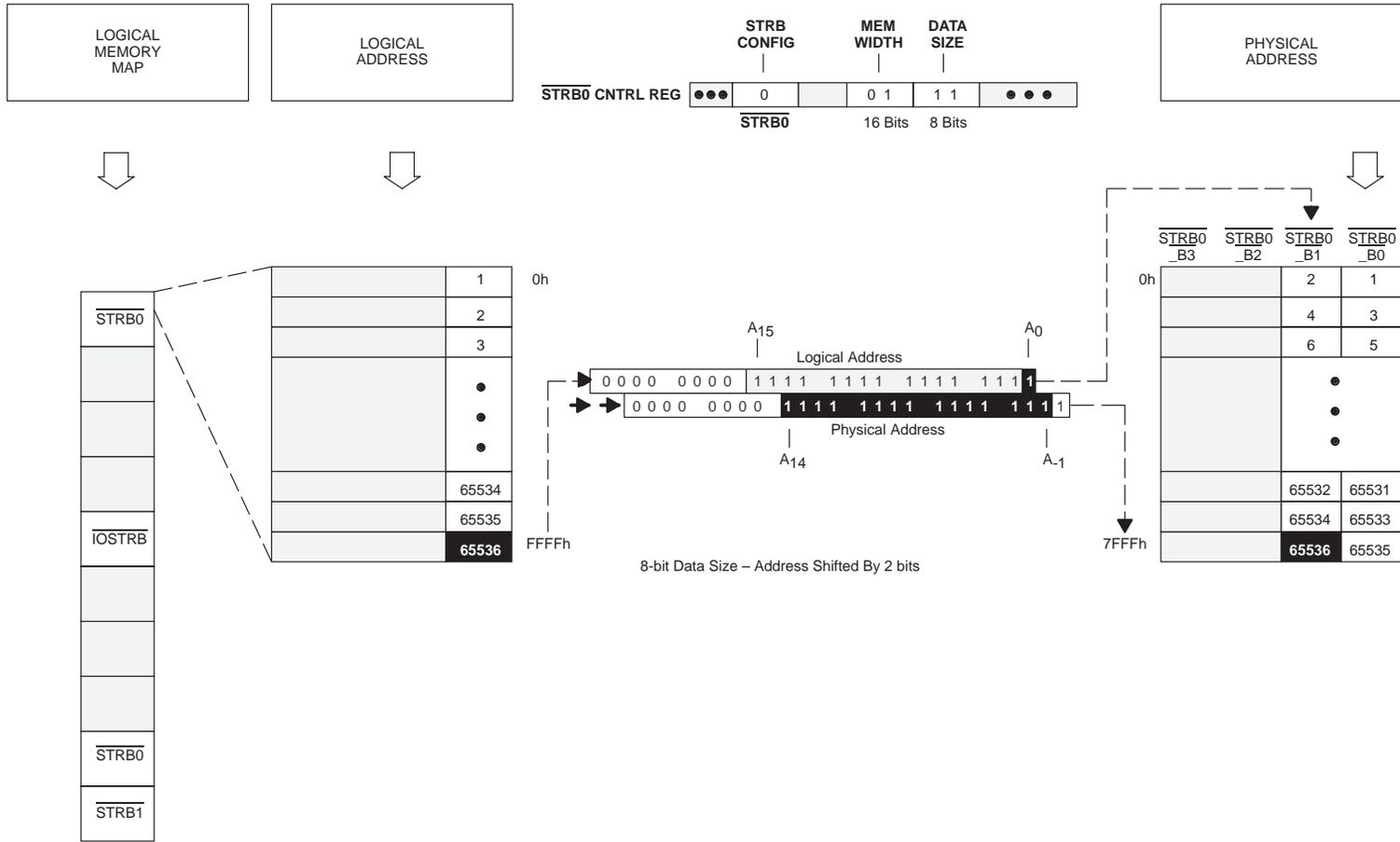
Figure 14. 16/8-Bit Memory Address Translation: Data Size < Memory Width
