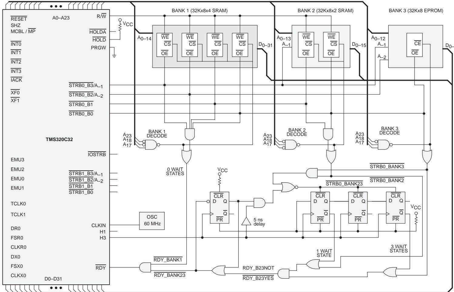
Figure 20.  $\overline{\text{RDY}}$  Signal Generation for  $\overline{\text{STRB0}}$  Cycles
