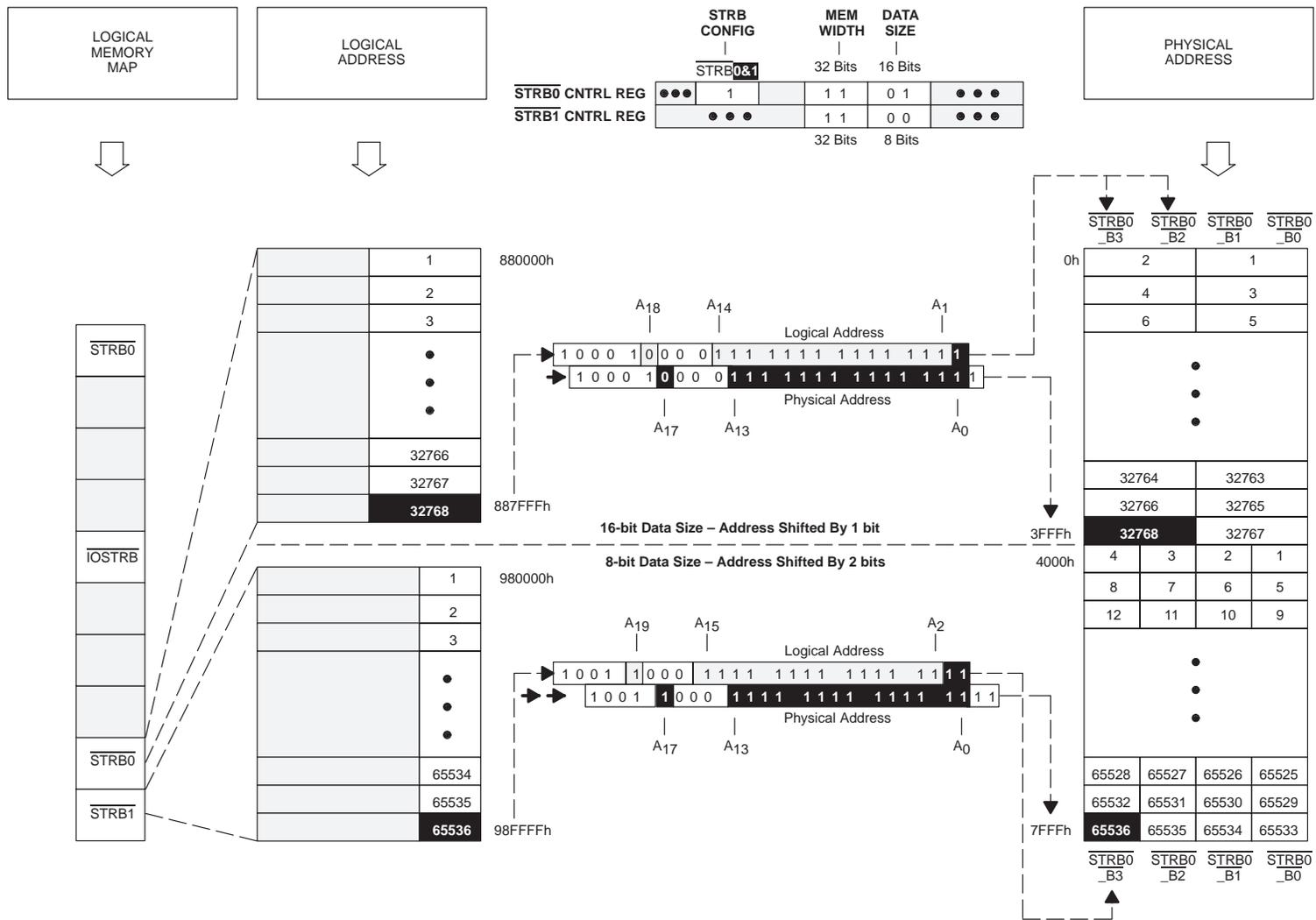
Figure 16. One Bank/Two Strobes Address Translation: Data Size = 16 and 8 Bits
