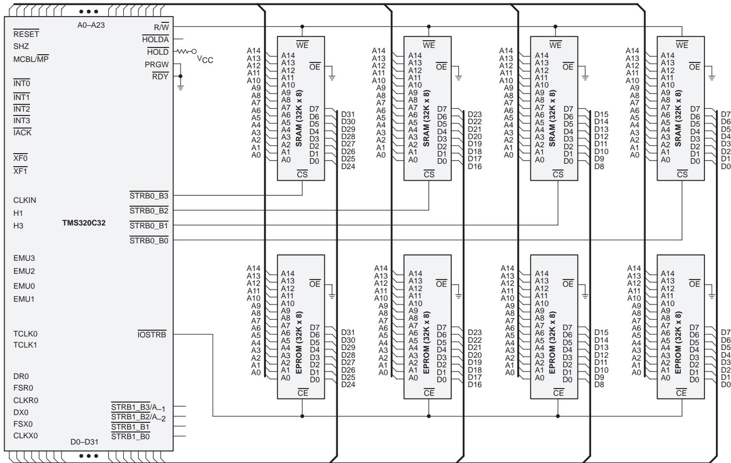
Figure 7. 32-Bit Memory Configuration ( $\overline{\text{STRB0}}$  and  $\overline{\text{IOSTRB}}$ )
