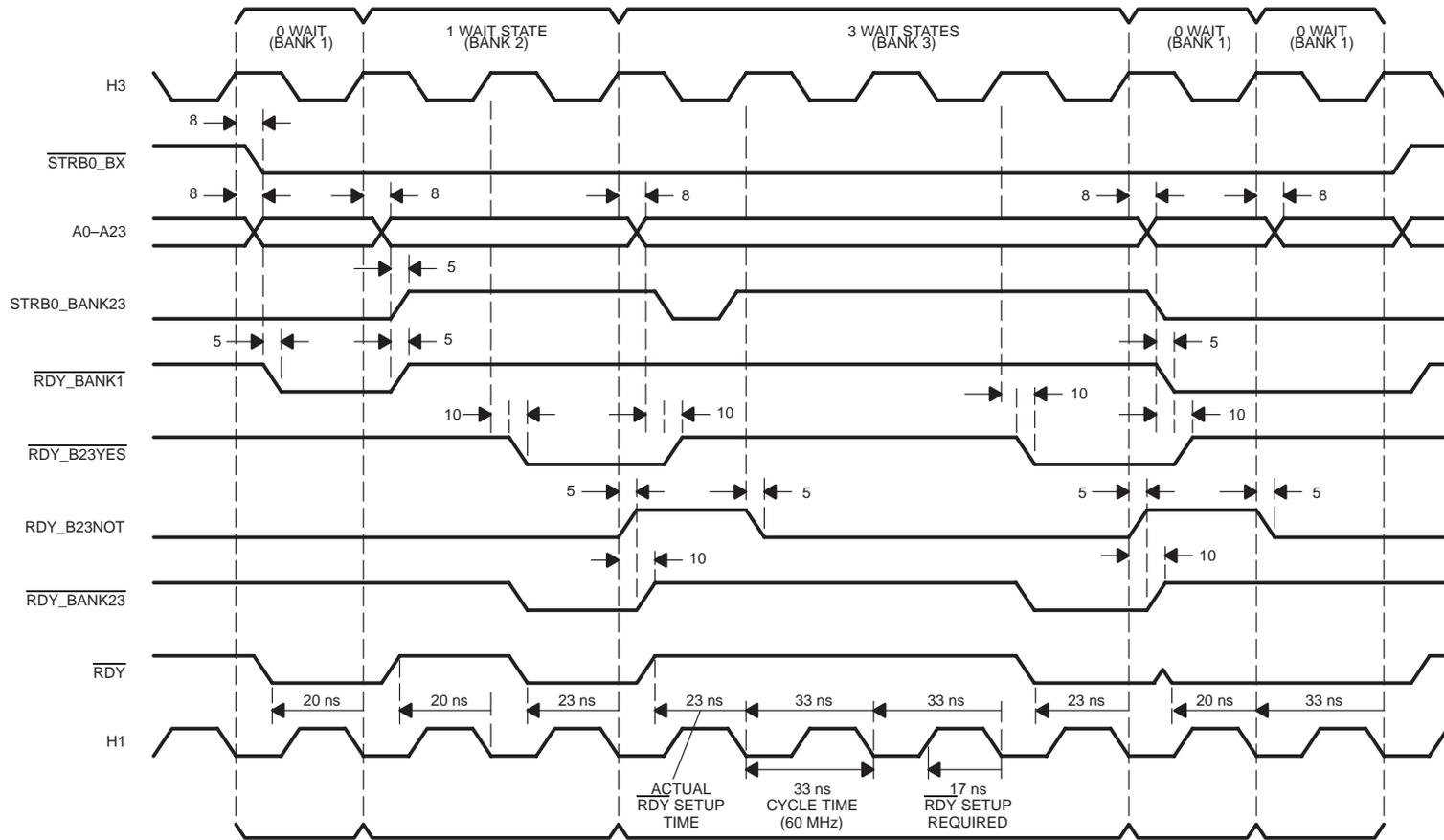
Figure 21.  $\overline{\text{RDY}}$  Signal Generation Timing Waveforms
