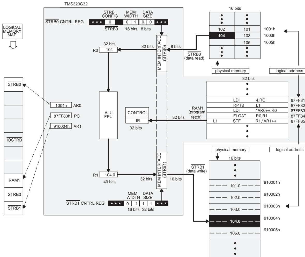
Figure 3.  $\overline{\text{STRB0}}$  and  $\overline{\text{STRB1}}$  Data Access: Data Size  $\neq$  Memory Width
