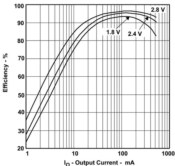
Figure 1. PWM Efficiency
