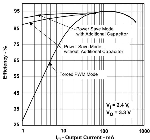
Figure 8. Efficiency Comparison
