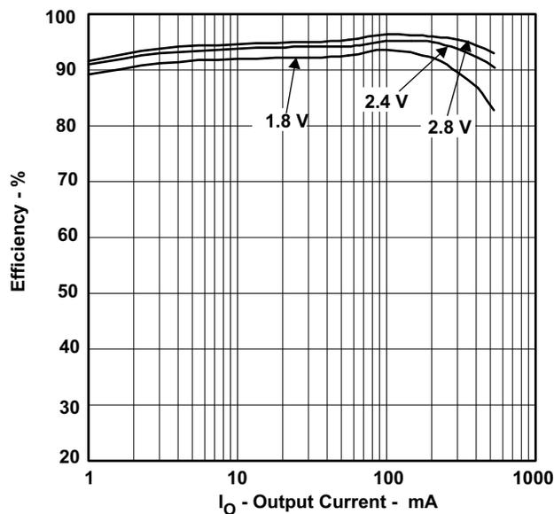
Figure 2. Power Save Mode Efficiency
