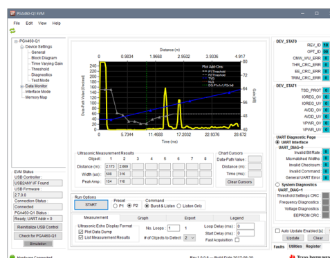
Figure 1. Typical Ultrasonic Decay Profile
