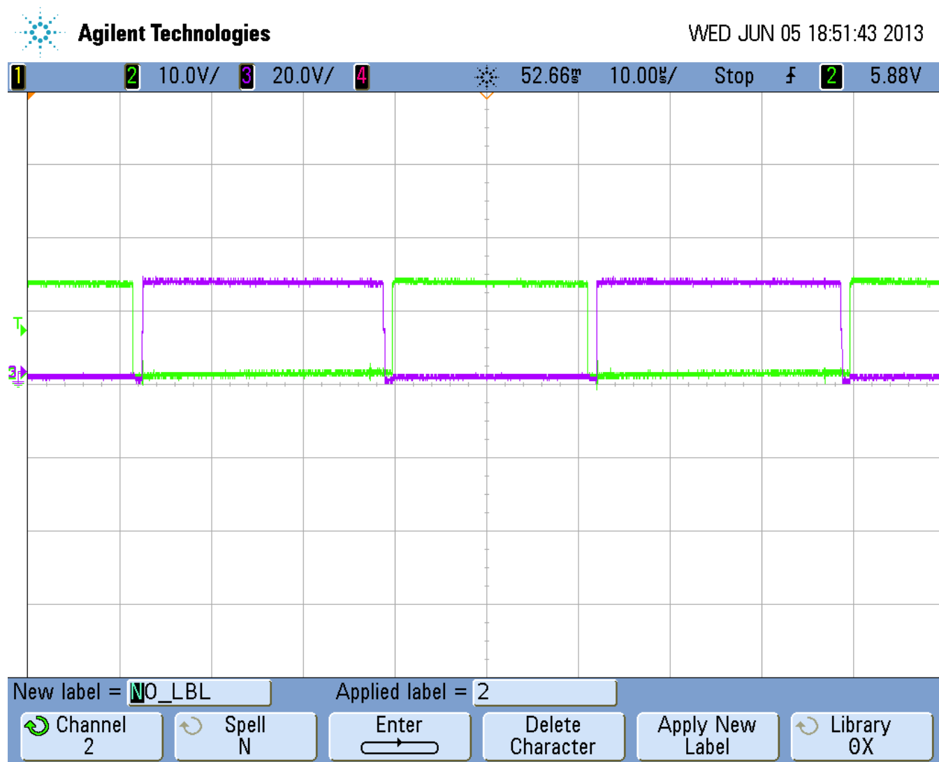
Figure 25. Dead Band between Complementary HOB and LOB Pair
