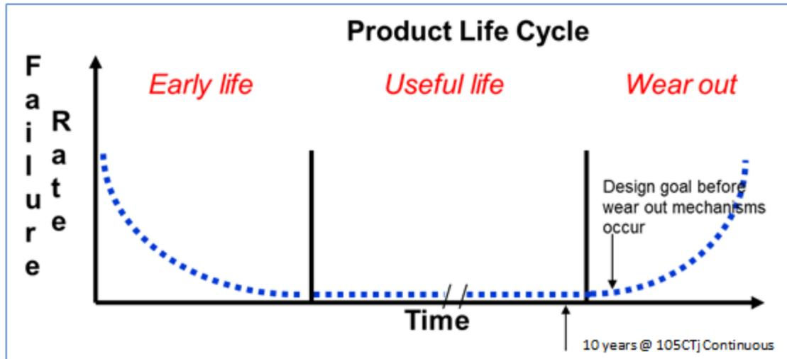
**Figure 1. Bathtub Curve Showing Different Stages of Reliability**
