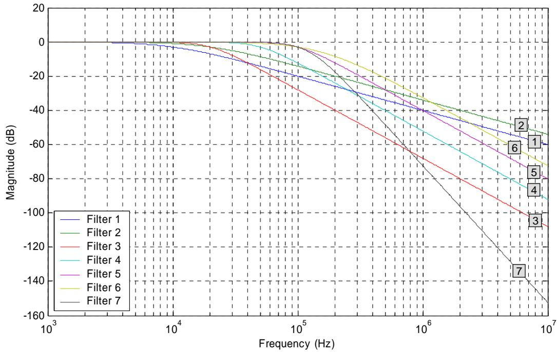
**Figure 8. Magnitude Response of the Analog Low-Pass Filters**
