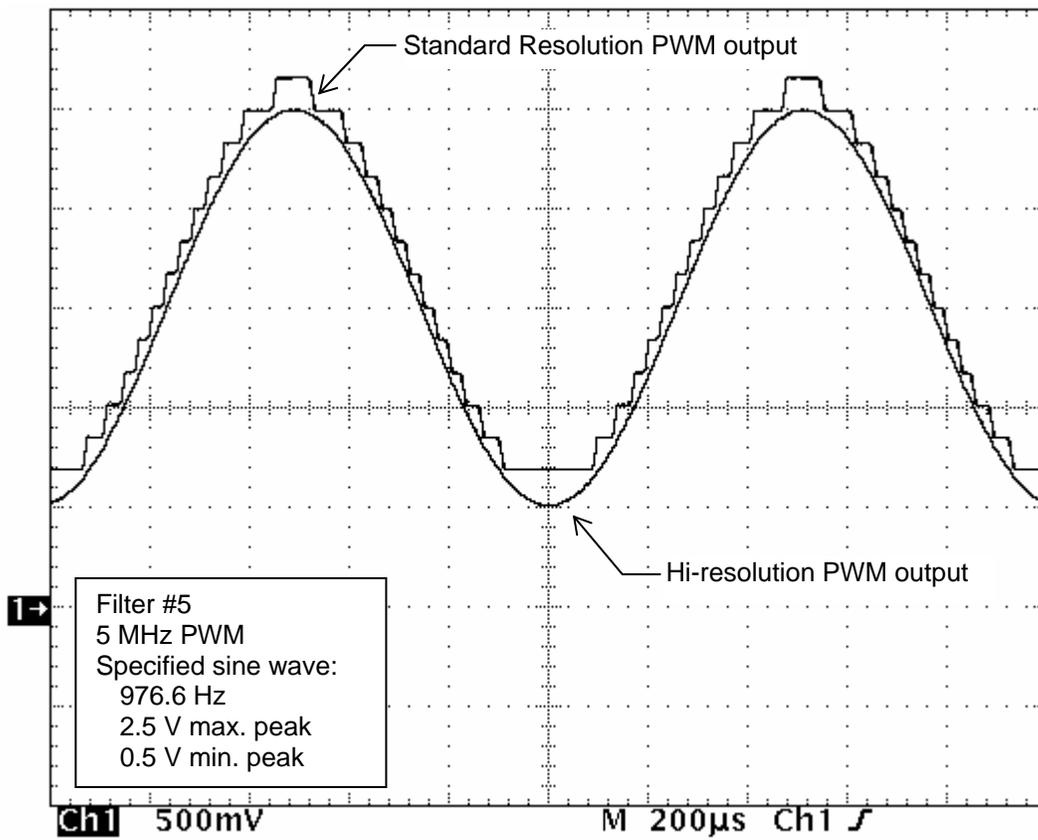
Figure 17. Filter #5 Output of PWM Sine Wave
