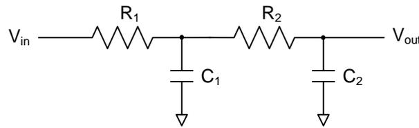
**Figure 6. 2<sup>nd</sup> Order Passive RC Low-Pass Filter Circuit**
