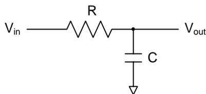
**Figure 5. 1<sup>st</sup> Order Passive Low-Pass Filter Circuit**
