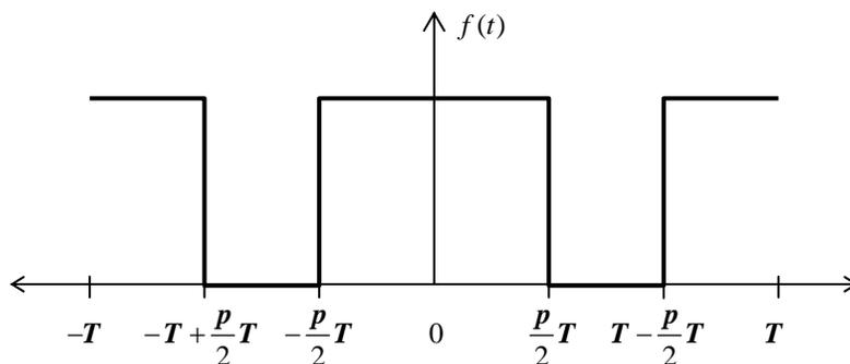
**Figure 3. PWM Signal Time-Shifted for Even Symmetry**
