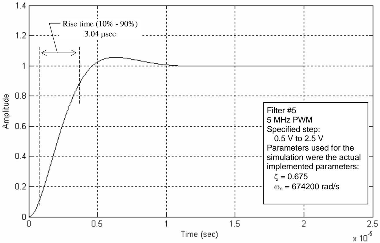
**Figure 19. Theoretical Filter #5 Unit Step Response (from Simulation)**
