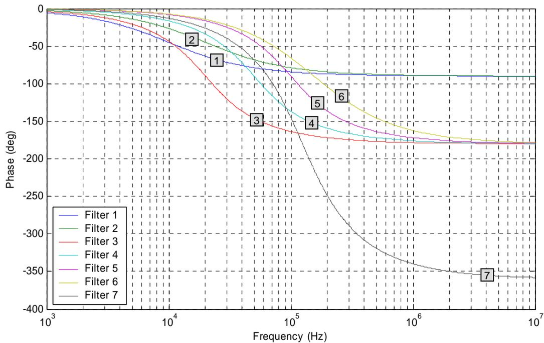
**Figure 9. Phase Response of Analog Low-Pass Filters**
