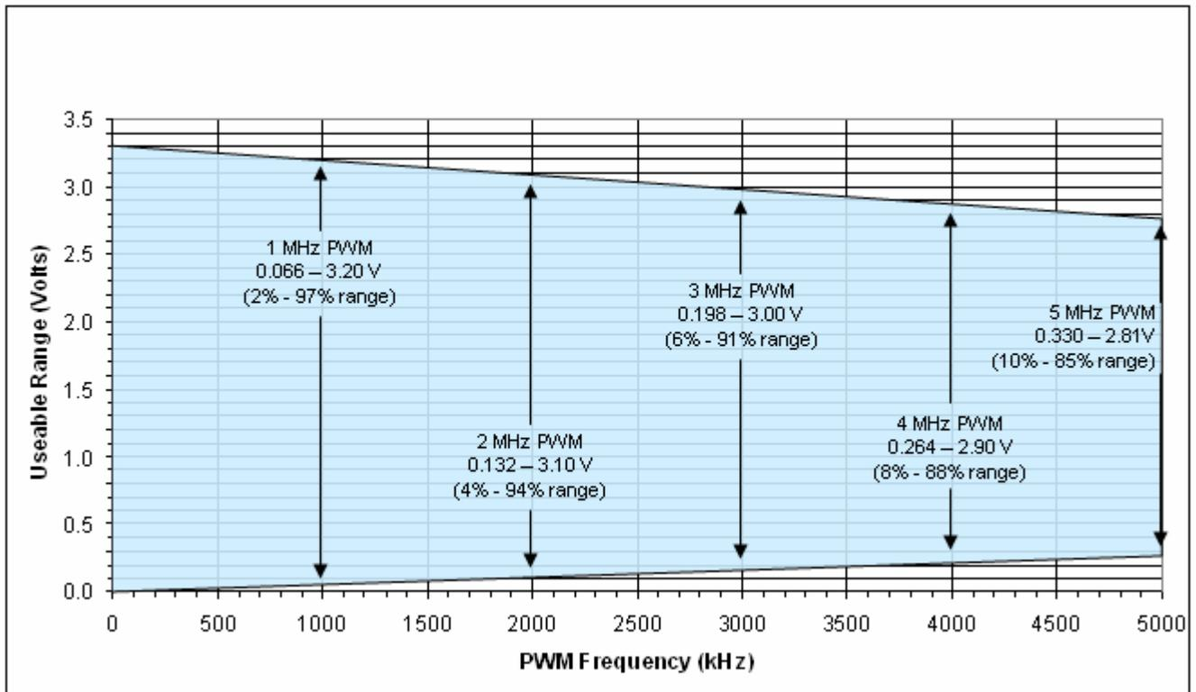
Figure 21. Effective Full-Scale D/A Range using HRPWM module
