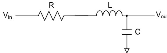
**Figure 7. 2<sup>nd</sup> Order Passive RLC Low-Pass Filter Circuit**
