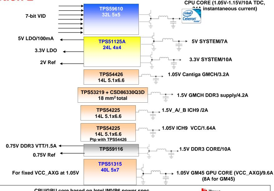
CPU/GPU core based on Intel IMVP6 power spec, rev.1.55, June 2009, pg.58
