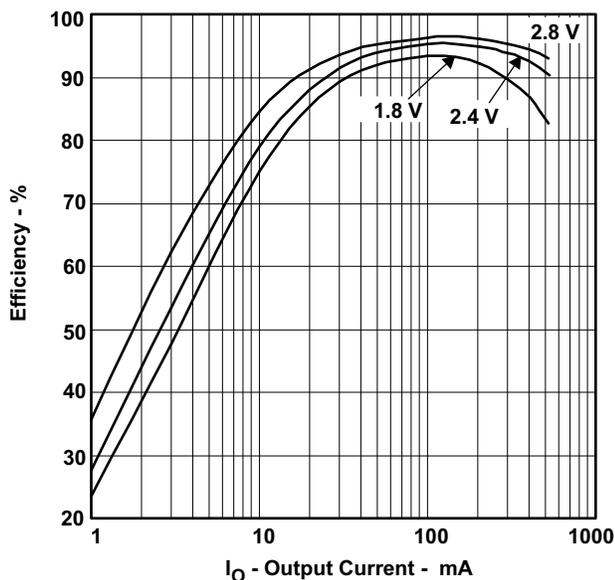
Figure 1. PWM Efficiency
