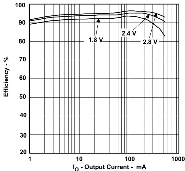
Figure 2. Power Save Mode Efficiency
