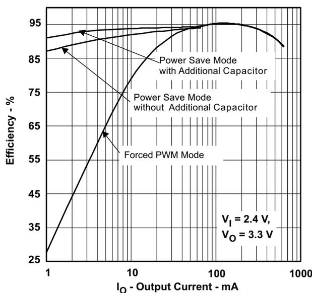
**Figure 8. Efficiency Comparison**
