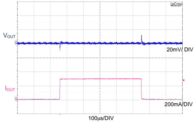
Figure 18. Load Transient in PWM Mode,  $V_{IN} = 3.8\text{ V}$ ,  $V_{OUT} = 2.5\text{ V}$ ,  $I_{OUT} = 0\text{ mA}$  to  $300\text{ mA}$ ,  $10\ \mu\text{s}$  Edge
