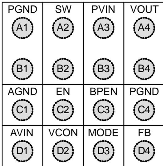
Figure 3. Bumps Face Down – Top-Through View
