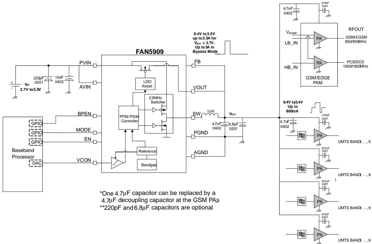
Figure 26. Typical Application Diagram with GSM/EDGE/WCDMA Transmitters
