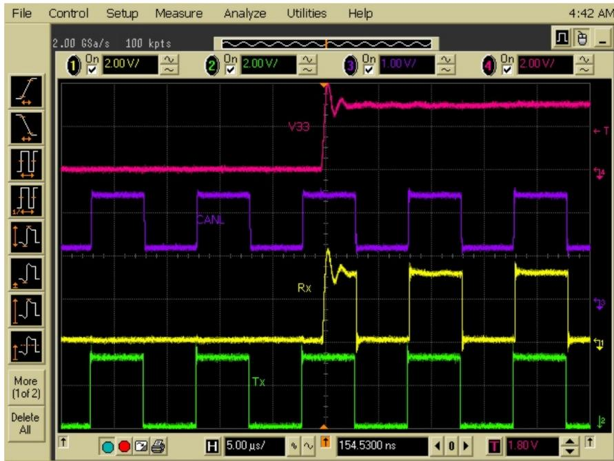
Figure 5. S is Close → V33 Transient at Recessive State (TxD = 1)
