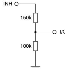
Figure 23. Simple 12 V-to-5 V Converter with Resistors
