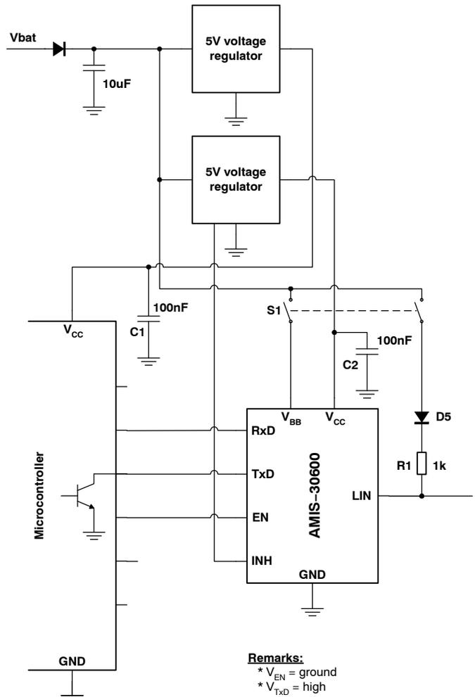
Figure 18. INH-pin Connected with 5 V Voltage Regulator
