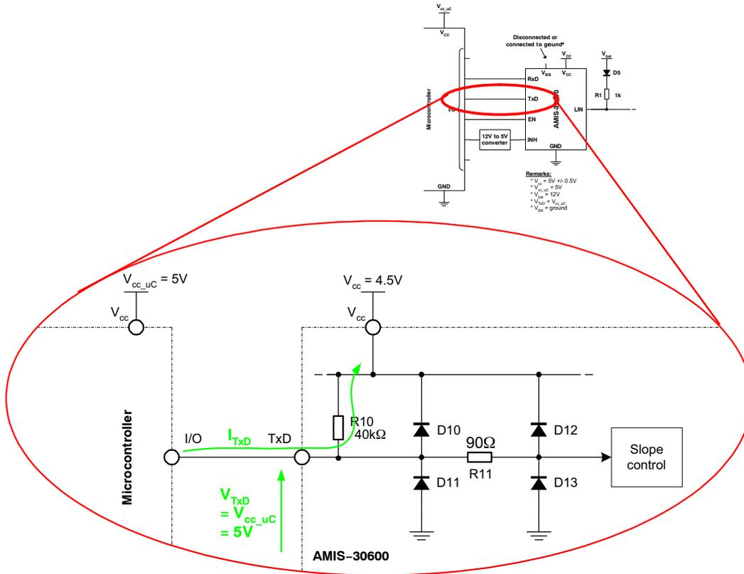
Figure 9.  $I_{TXD}$  when ESD Protection Diodes Don't Conduct<sup>7</sup>
