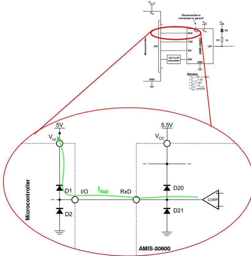
Figure 10. ESD Protection Diode D1 Conducts<sup>8</sup>
