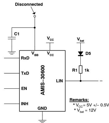
**Figure 12. Decoupling Capacitor Present when  $V_{BB}$  is Disconnected**
