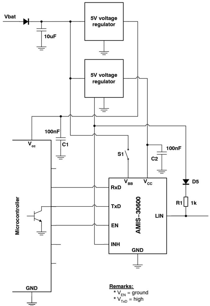
**Figure 19. INH-Pin used to Disconnect LIN Pullup Resistor**
