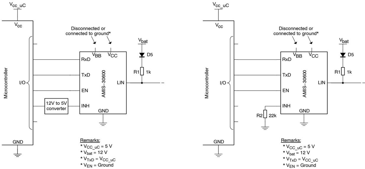
**Figure 2.  $V_{BB}$  Disconnected or Connected to Ground**
