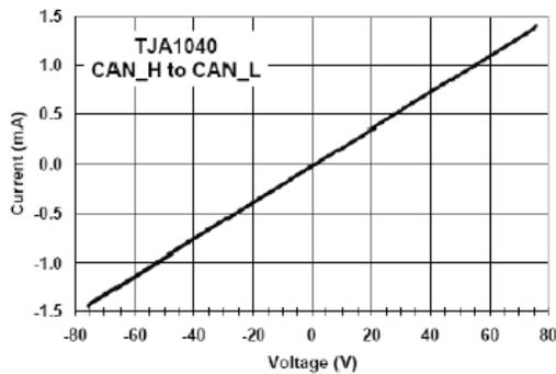
Figure 5. The impedance between the CAN\_L and CAN\_H data lines is 55 KΩ.
