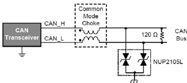
**Figure 11. TVS diodes and a common mode choke filter create an effective CAN transceiver surge protection circuit.**
