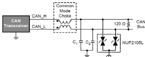
**Figure 14. Capacitors  $C_1$  and  $C_2$  can be used to filter high frequency noise signals.**
