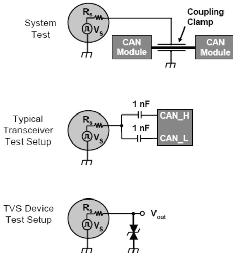
Figure 6. Surge test configurations for a system, transceiver IC and a TVS device.
