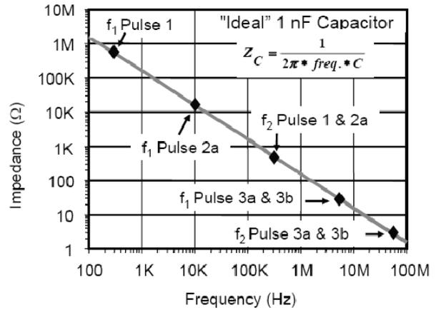
Figure 8. A 1.0 nF capacitor has significant impedance at the frequencies contained in the ISO 7637-2 pulse 1 and 2a surge tests.
