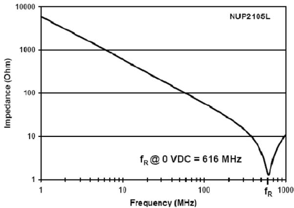
**Figure 13. The NUP2105L functions as a capacitor at frequencies below the resonant frequency ( $f_R$ ); however, the inductance term must be included at frequencies greater than  $f_R$ .**
