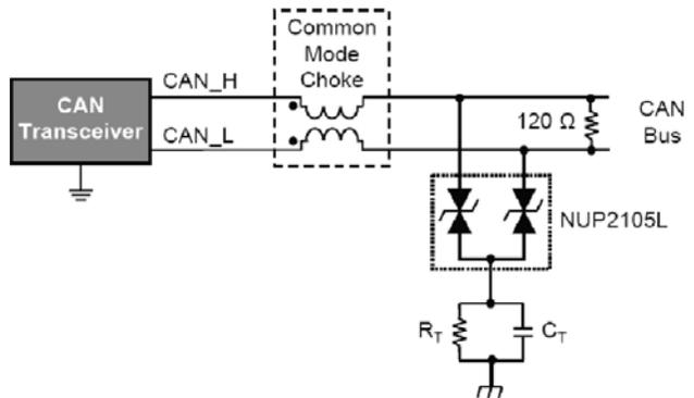
**Figure 12. Adding a RC network on the ground connection of the TVS diode array increases the surge immunity by limiting the current through the NUP2105L diodes.**
