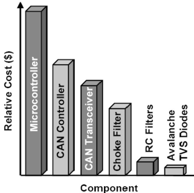
Figure 1. TVS diodes are a low cost solution to increase the surge immunity level of a CAN network.
