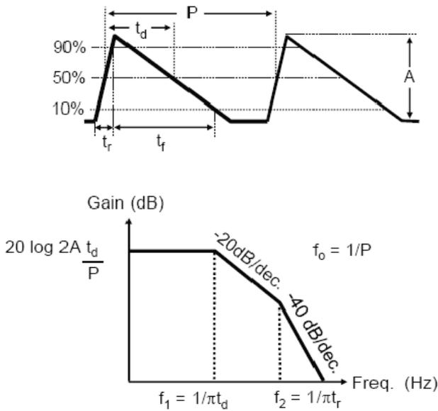
Figure 7. The frequency spectrum of the ISO 7637 surge pulses can be estimated from the rise time ( $t_r$ ) and pulse duration ( $t_d$ ).
