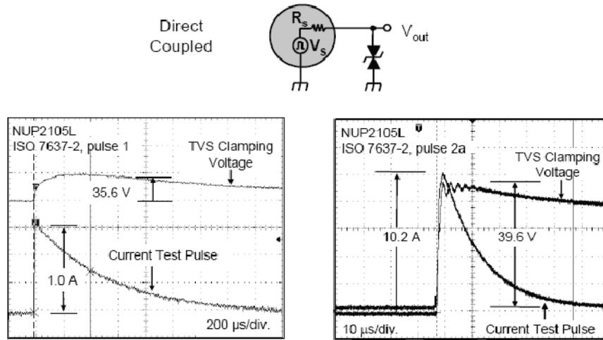
**Figure 9. The NUP2105L clamps the pulse 1 and 2a surge pulses to 35.6 V and 39.6 V, respectively.**
