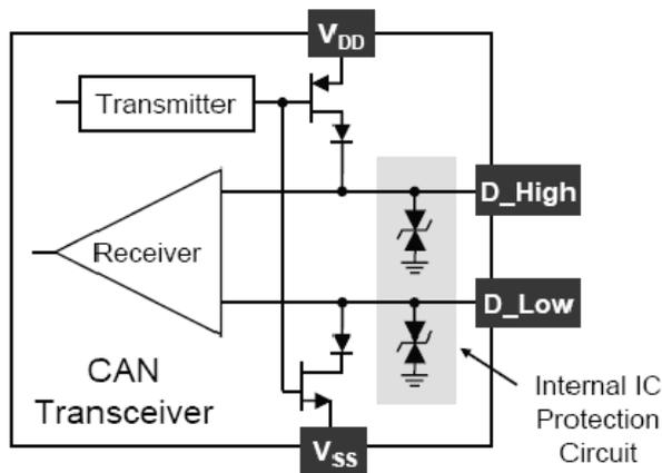
**Figure 2. Zener diodes are a popular choice for internal TVS protection circuits.**
