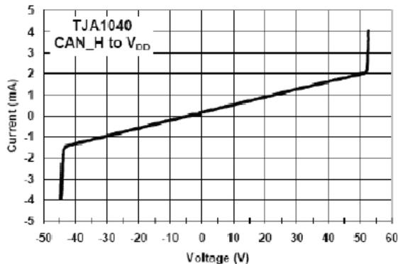
**Figure 3. The current versus voltage graphs between the CAN data lines and ground show that the protection circuits are equivalent to two bidirectional Zeners with a breakdown voltage of approximately  $-40$  V/ $+50$  V.**
