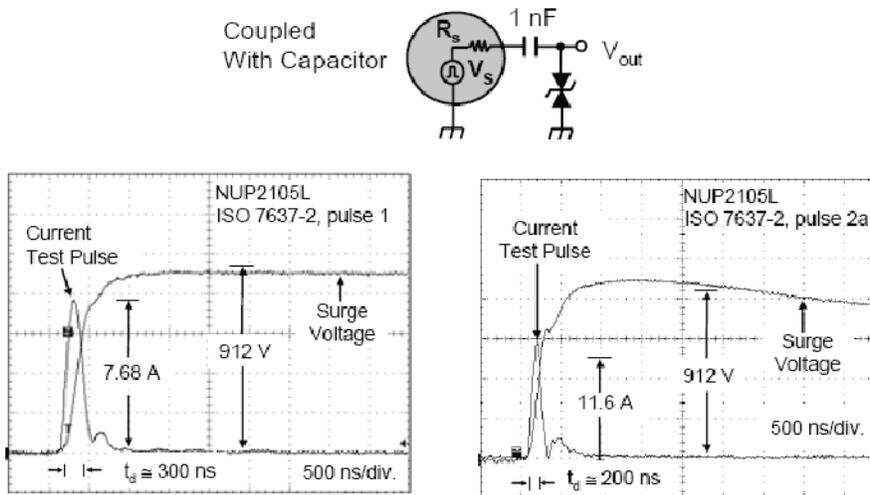
**Figure 10. A 1.0 nF coupling capacitor reduces the energy of the pulse 1 and 2a tests by shortening the duration of the surge pulses to 300 and 180 ns, respectively.**
