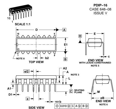
STYLE 1: STYLE 2: PIN 1. CATHODE CATHODE PIN 1. 2. COMMON DRAIN COMMON DRAIN 2. 3. CATHODE 3. COMMON DRAIN COMMON DRAIN COMMON DRAIN 4. 5. CATHODE 4. CATHODE 5. 6. CATHODE 6. COMMON DRAIN 7. CATHODE 7. COMMON DRAIN CATHODE COMMON DRAIN 8. 9. 8. 9. ANODE GATE 10. ANODE 10. SOURCE 11. 12. ANODE ANODE 11. 12. GATE SOURCE 13. ANODE 13. GATE 14. 15. ANODE ANODE 14. 15. SOURCE GATE 16. ANODE 16. SOURCE
