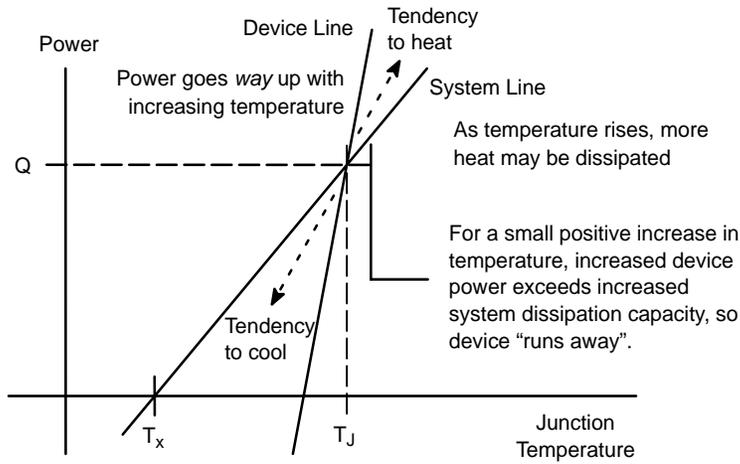
**Figure 4. Operating Point of Thermal System where Power Increases with Temperature, Slopes Unfavorable**
