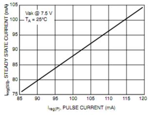
Figure 7. I<sub>Reg(SS)</sub> vs. I<sub>Reg(P)</sub>
