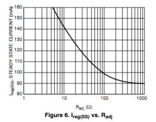
Notice how flat the  $R_{adj}$  value is as it gets to 90mA. This means that initially the  $R_{adj}$  pin can be left open. If the overall solution gets too hot and the CCR reduced the current through the LEDs to the point where they are not being driven near 100 mA then a resistor can be added to boost the current. Since no real test can duplicate the effects of every LED tube or LED bulb it is recommended to first build a prototype then modify the  $R_{adj}$  value. The  $R_{adj}$  can be
