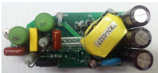
Figure 2. Top View (Dimensions: 34.5 mm (W) x 75 mm (L) x 20 mm (H))
