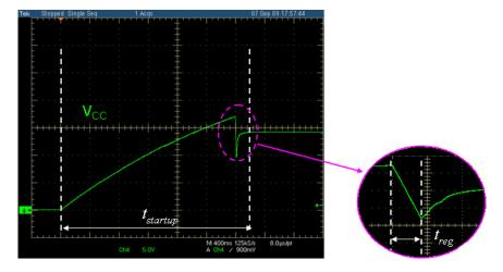
Figure 8. V<sub>CC</sub> Waveform during Startup
