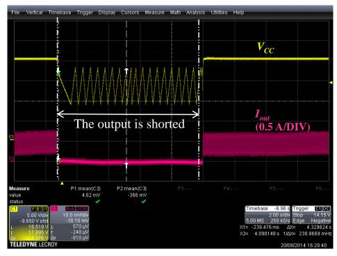
Figure 14. The System Enters a Safe Low Duty-ratio Burst Mode when the Output is Shorted (the LED Driver Output is Shorted for about 10 s for this Test)
