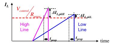
Figure 5. Propagation Delay Effect on Peak Current
