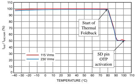
Figure 10. LED Current Characteristics over the Temperature Range
