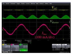
Figure 12. Current Waveform at 115 V rms
