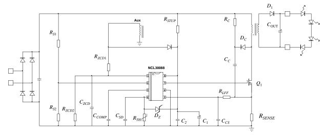
Figure 2. Basic Schematic
