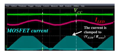
Figure 1. Current Over-current Limitation (V<sub>ILIM</sub> is the Over-current Threshold, R<sub>sense</sub> the Current Sense Resistor)
