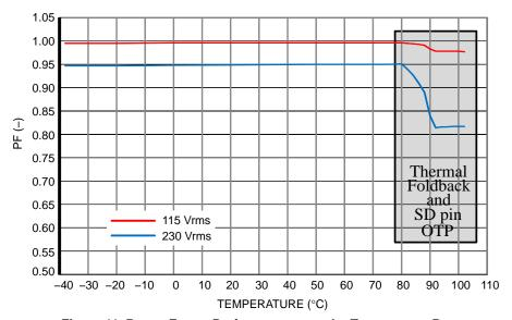
Figure 11. Power Factor Performance over the Temperature Range
