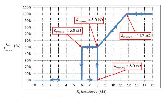
Figure 6. Thermal Foldback Characteristics and Over-temperature Protection
