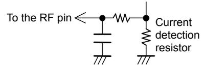
High-precision detection can be implemented by connecting the lines from the RF and RFGND pins close to the two terminal of the current detection resistor  $R_f$ .
