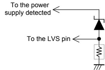
If the LVS pin is left open, the internal pull-down resistor will result in the IC seeing a ground level input, and the output will be turned off. Therefore, a voltage in excess of the LVS circuit clear voltage (about 4.35 V) must be applied to the LVS pin if the application does not use the undervoltage protection circuit. The maximum rating for the LVS pin applied voltage is 18 V.
