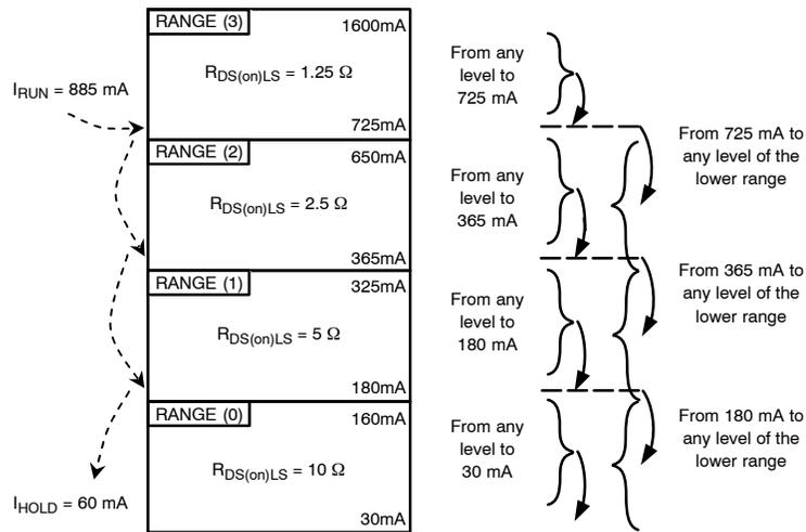
Figure 3. Suggested Current Level Switching with the 52x\*
