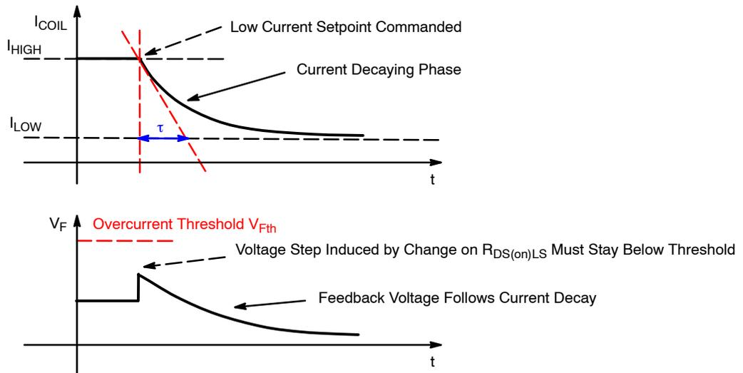
**Figure 2. Coil Current Decay when Low Levels are Commanded**
