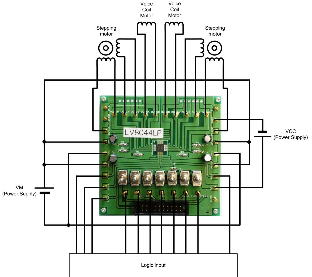
(Circuit diagram of the evaluation board)
