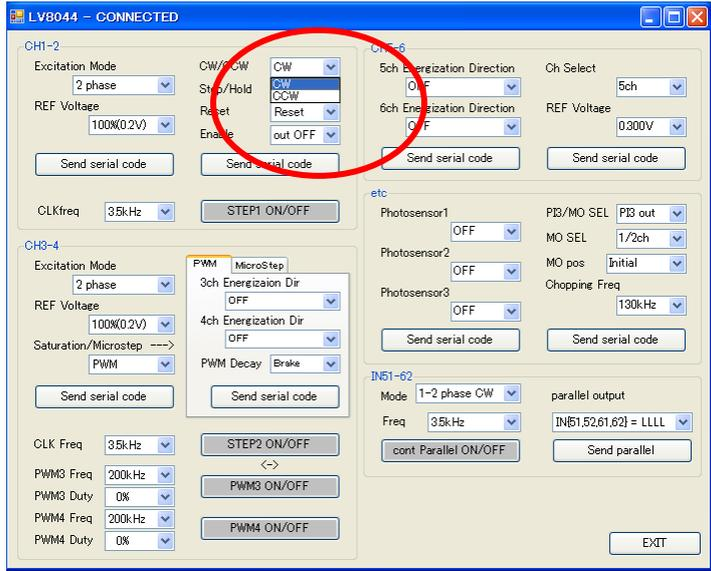
Also, when the stepper motor is driven, the frequency of the reference clock signal “STEP1” is set. And, it is turned on / off by using the “STEP1 ON/OFF” button.
