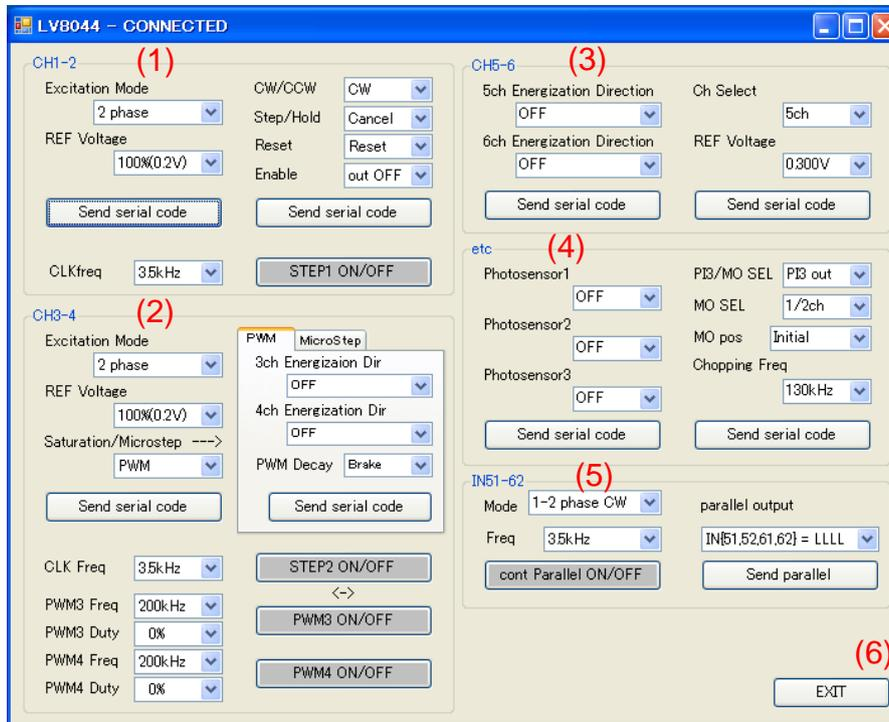
(1) “CH1-2” setting field : the serial signal to drive the stepper motor between CH1 and CH2 is set.
