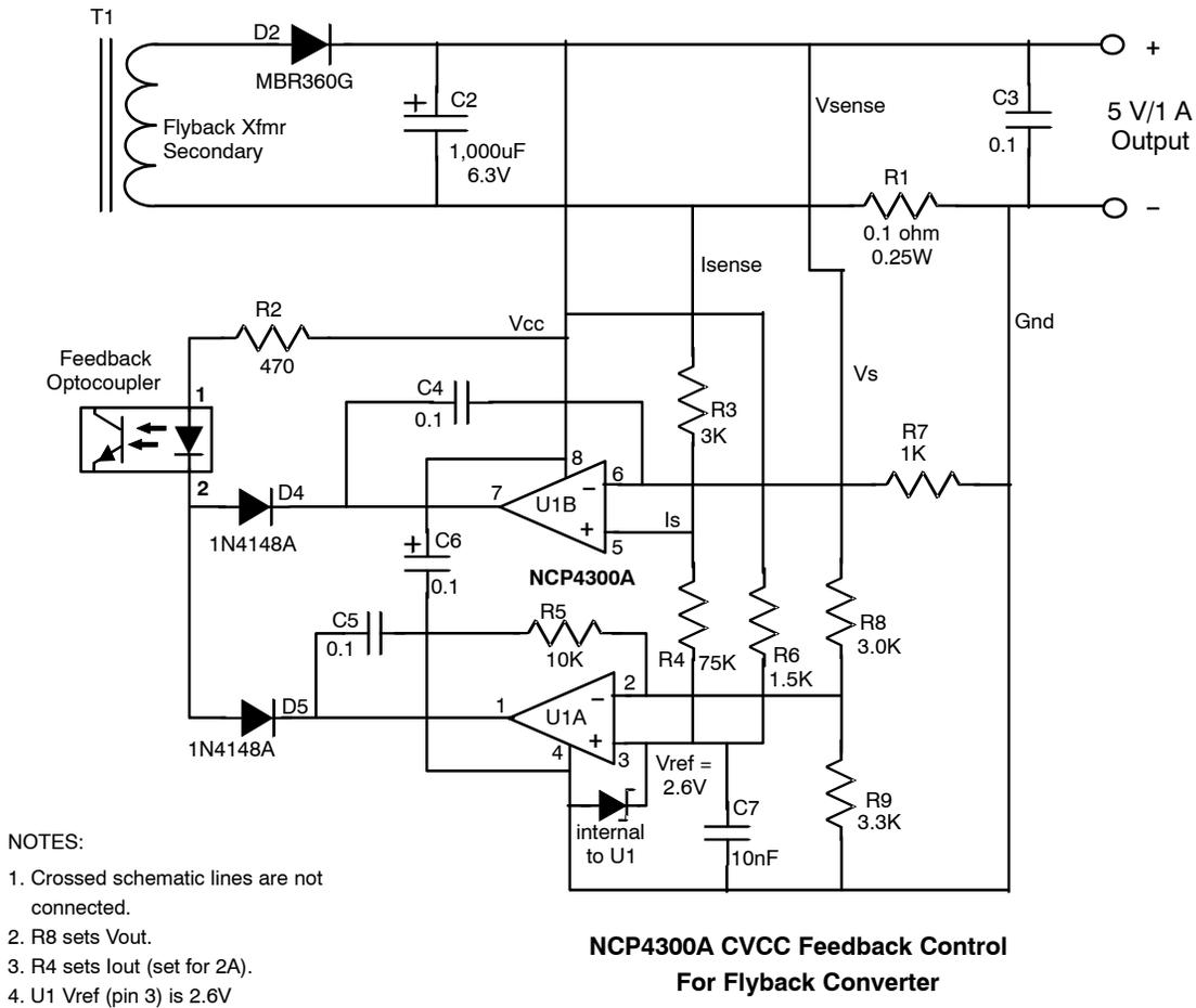
**Figure 3. A Possible Solution for CVCC Charger Efficiency Improvement**
