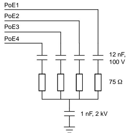
Figure 1. Bob Smith Termination for Power-over-Ethernet Circuits
