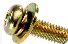
Figure 6. SEMS Screw (Size M3, Spring Washer 5.0Φ, Plain Washer 7.5Φ)
