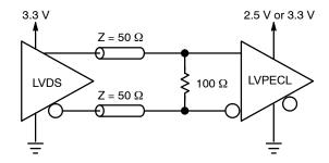
Figure 17. Interfacing LVDS to LVPECL
