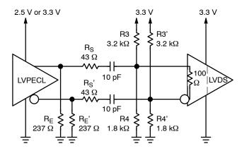
Figure 6. Capacitive Coupling LVPECL to LVDS
