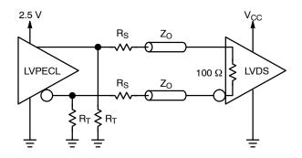
Figure 12. Interfacing 2.5 V LVPECL to LVDS with Series  ${\rm R}_{\rm S}$  and Internal 100  $\Omega$  Termination Resistor
