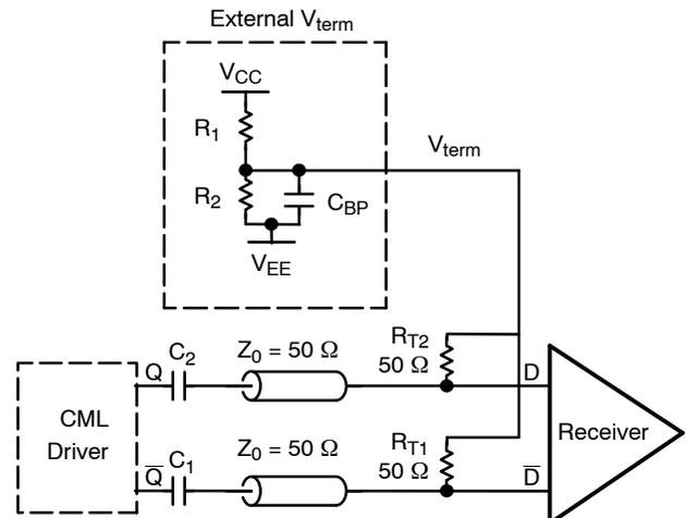
Figure 8. Typical V<sub>term</sub> Supply Divider Network
