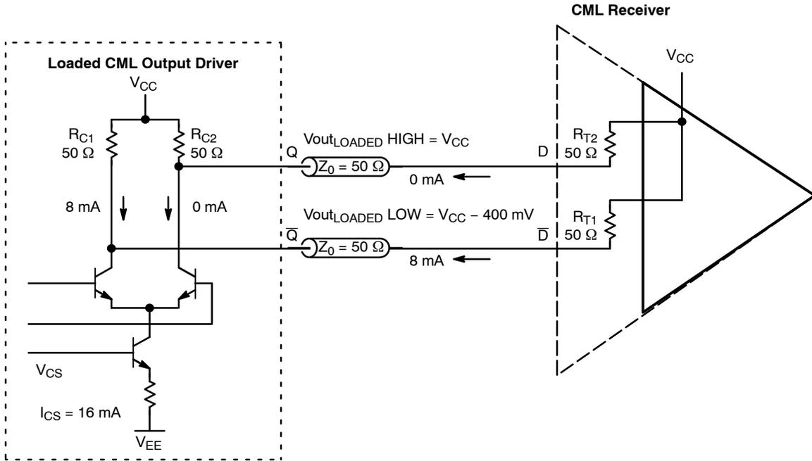
Figure 5. CML Output (with Direct Connect Load Termination of 50 Ω per line to V<sub>CC</sub>), Currents and Levels (Q HIGH, Q̄ LOW)
