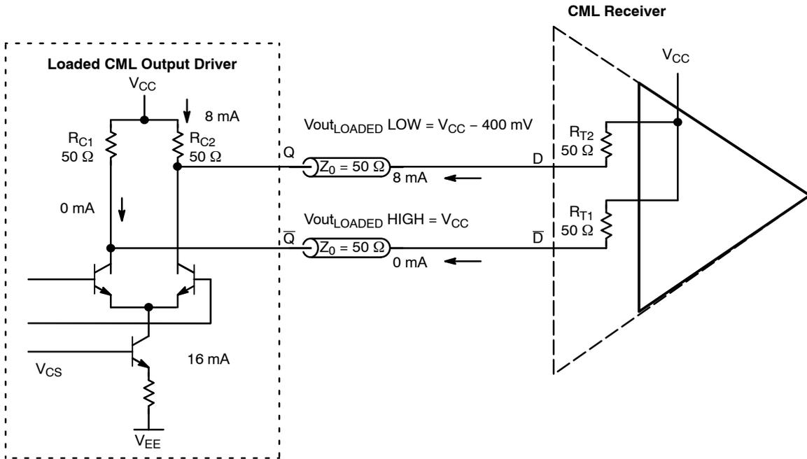
Figure 6. CML Output (with Direct Connect Load Termination of 50 Ω per line to V<sub>CC</sub>), Currents and Levels (Q LOW, Q̄ HIGH)
