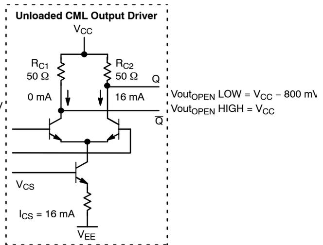
**Figure 4. CML Open Output Driver Currents and Levels (Q LOW,  $\bar{Q}$  HIGH)**
