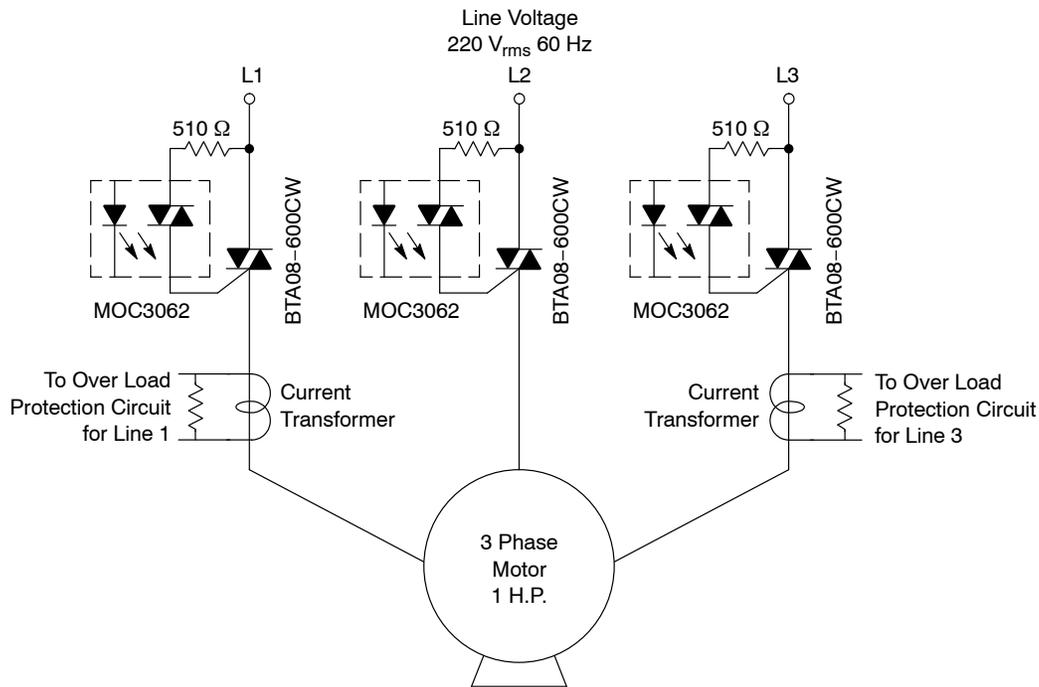
**Diagram 1** shows how three triacs BTA08-600CW3G or BTB08-600CW3G (Ref: BTA08-600CW) substitute the mechanical contacts of the conventional magnetic starter (shown previously) for supplying the power to the three phase 1HP motor once the triacs are triggered.
