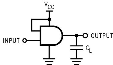
C<sub>L</sub> includes load and stray capacitance
