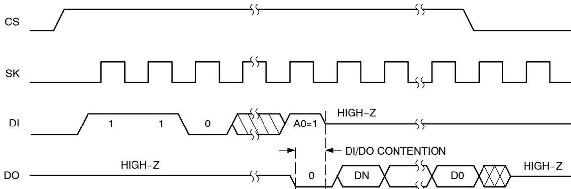
Figure 1. DI/DO Contention Timing During Read Cycle
