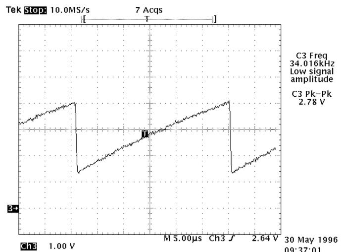
Figure 2. Controller Oscillator Voltage Ramp
