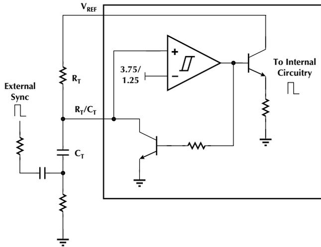
**Figure 3. Controller Oscillator Circuit (with External Synchronization)**
