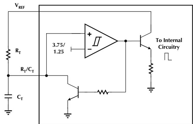
Figure 1. Typical Controller Oscillator Circuit
