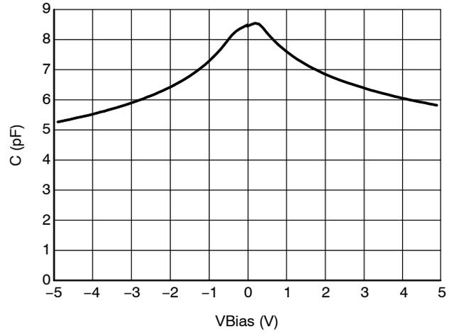
Figure 4. CV Characteristics
