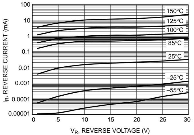
Figure 6. Leakage Current
