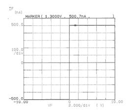
Figure 6. Short Circuit IV Caused by Improper Mounting
