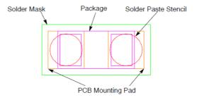
Figure 7. Recommended Mounting Pattern
