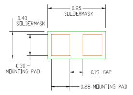
Figure 9. Recommended Mounting Pattern
