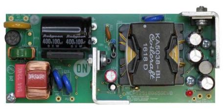
Figure 5. Evolution Board Photo – Top Side
