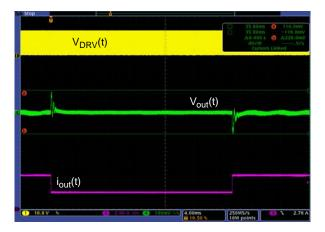
Figure 15. Transition Response –  $I_{OUT}$  = 1.75 A to 3.5 A,  $V_{IN}$  = 230 V, Slew Rate 0.5 A/ $\mu s$
