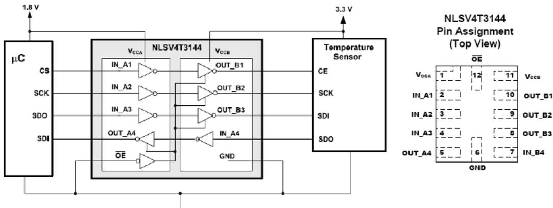
Figure 7. The Three Input / One Output Circuit Topology of the NLSV4T3144 Matches the I/O Structure of the Four Wire SPI Bus
