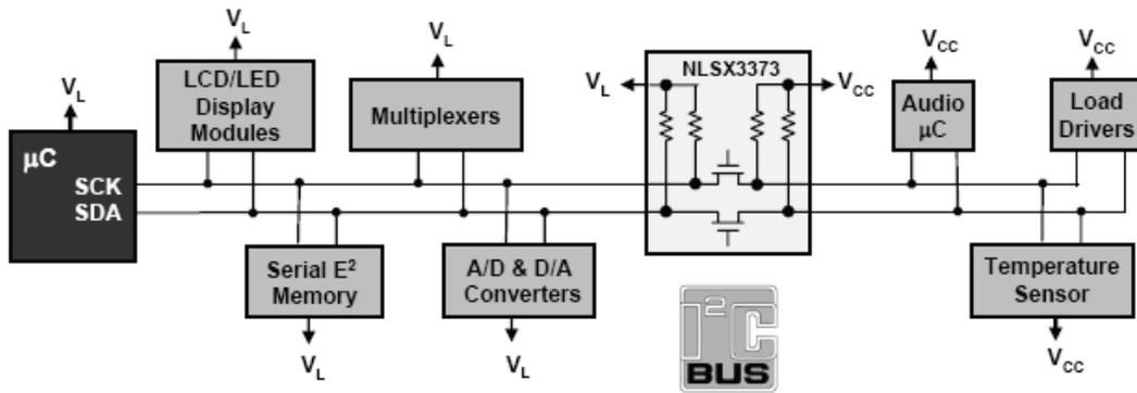
**Figure 2. Open-Drain Autosense Voltage Translators Connect a Processor to I<sup>2</sup>C Bus Peripherals that have Different Operating Voltages**
