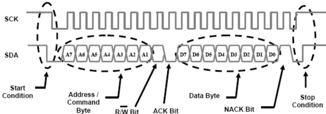
**Figure 3. The I<sup>2</sup>C Serial Communication Frame Consists of Serial Clock (SCK) and Serial Data (SDA) Signal Lines**
