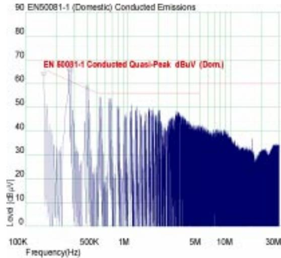
Figure 6. X2 47 n Capacitor at Input
