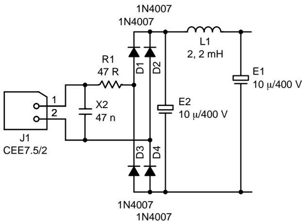
Figure 7. Complete EMI Filter
