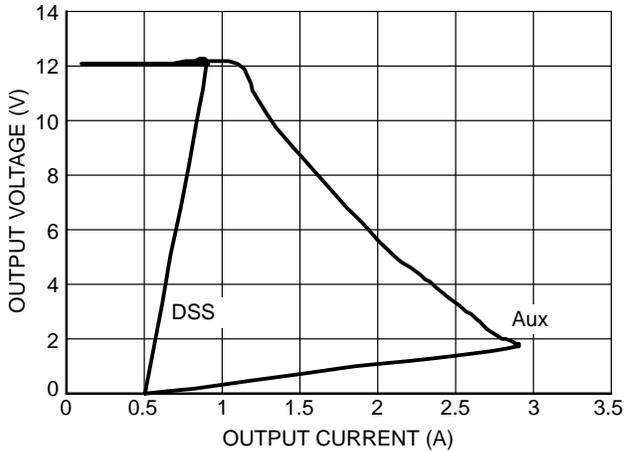
**Figure 4. Vout vs Iout (330 Vdc)
