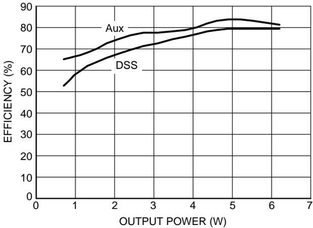
**Figure 2. Efficiency vs Power, Vin = 330 Vdc
