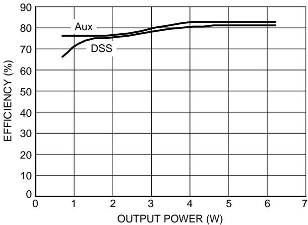
**Figure 3. Efficiency vs Power, Vin = 120 Vdc
