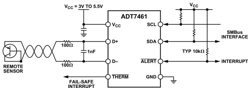
Figure 1. Circuit Diagram
