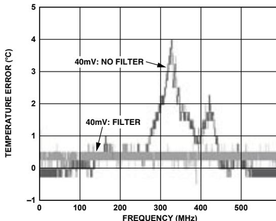
Figure 2. Effect of Filter on 40 mV Noise
