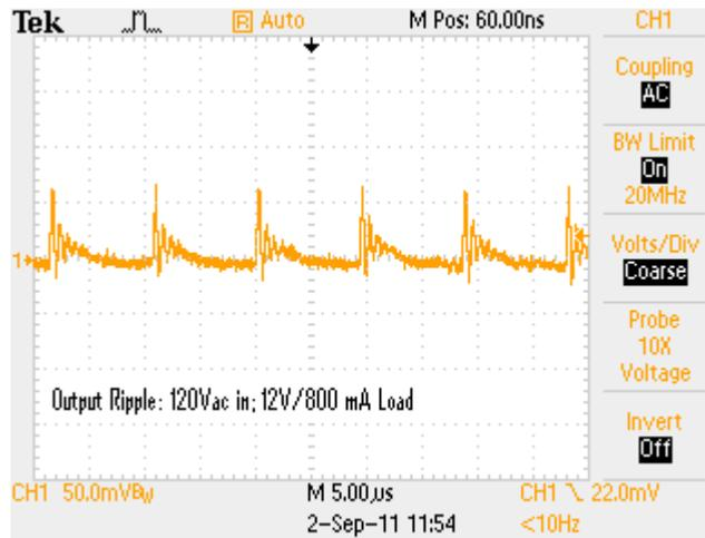
Figure 2. Full Load Output Ripple @ 120 Vac Input
