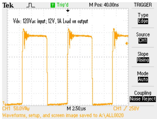
Figure 3. MOSFET Drain Voltage (120 Vac Input, 12 V, 1 A Load on Output)
