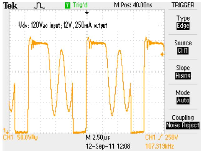
Figure 4. MOSFET Drain Voltage (120 Vac Input, 12 V, 250 mA Output)
