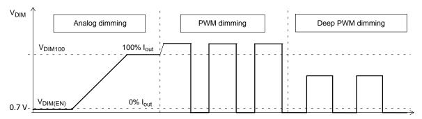
Figure 10. Analog / PWM Dimming
