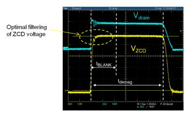
Figure 6. Optimal Filtering of ZCD Pin Voltage
