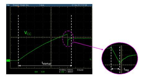
Figure 12. V<sub>CC</sub> Waveform during Startup
