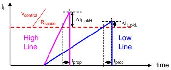
Figure 8. Propagation Delay Effect on Peak Current
