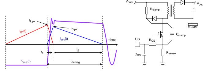
Figure 1. Fly-back Currents and Auxiliary Winding Voltage in DCM
