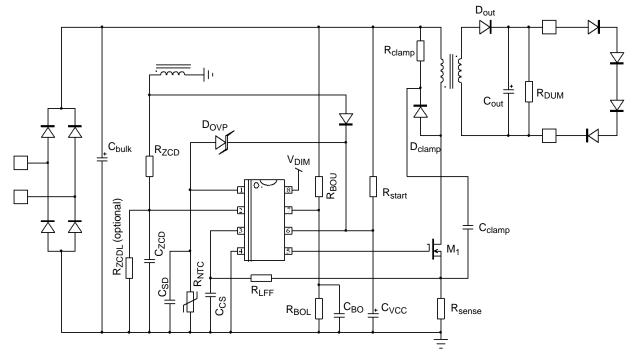
Figure 7. Generic Application Schematic
