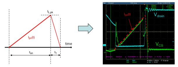
Figure 3. Current Sense Voltage Waveform for an Accurate Current Regulation
