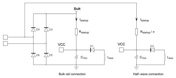
Figure 11. The Startup Resistor can be Connected to the Bulk Rail or to the Half Wave
