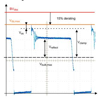
Figure 13. MOSFET Drain-source Voltage at High Line
