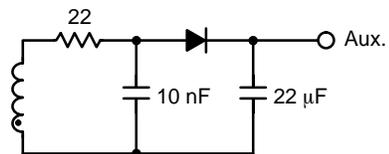
**Figure 5. A Resistor and a Capacitor Can Integrate the Perfidious Leakage Inductance**
