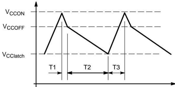
**Figure 20. V<sub>CC</sub> Waveform when the Optocoupler is Lost, e.g. During an Overload.**
