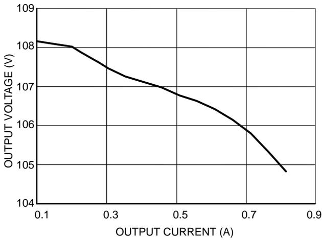
Figure 25. Static Load Response at 325 VDC Input
