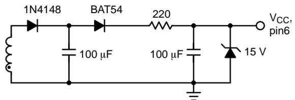
**Figure 6. This Configuration Ensures Self-Supply in Standby and Prevents V<sub>CC</sub> from Exceeding the 16 V Maximum Rating**
