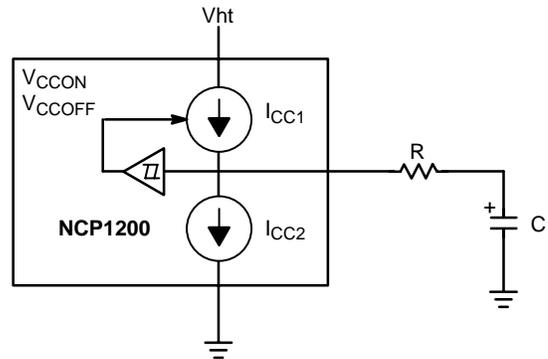
**Figure 21. Inserting a Single Resistor in Series with the V<sub>CC</sub> Capacitor Help Reducing the Burst Duty-Cycle**
